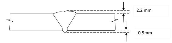
Weld reinforcement allowed by Code for Visual Inspection of 12.4mm wall thickness groove weld in butt joint
