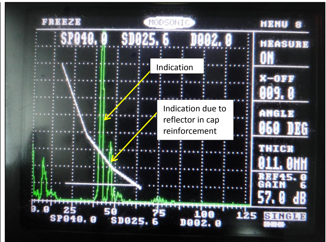
Lack of fusion defect at fusion face in a branch member @ DAC (45 + 12 dB)
