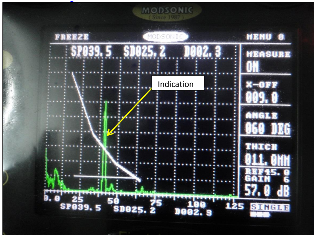
Vertically oriented lack of fusion defects at fusion face in a main member @ DAC (45 + 12 dB)
