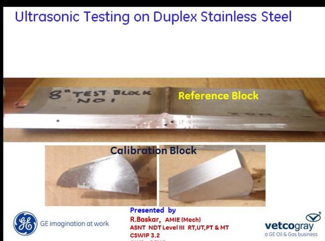
**Ultrasonic Testing on Duplex Stainless Steel**
